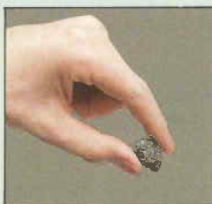
These very hard materials are used in the barrier to blunt drills and discs.
